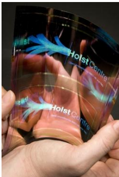
Figure 2 - Holst Centre develops flexible OLED on transparent substrates
