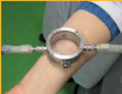
Fig. 3: Gas collection chamber (built by the University Hospital of the RWTH Aachen).
