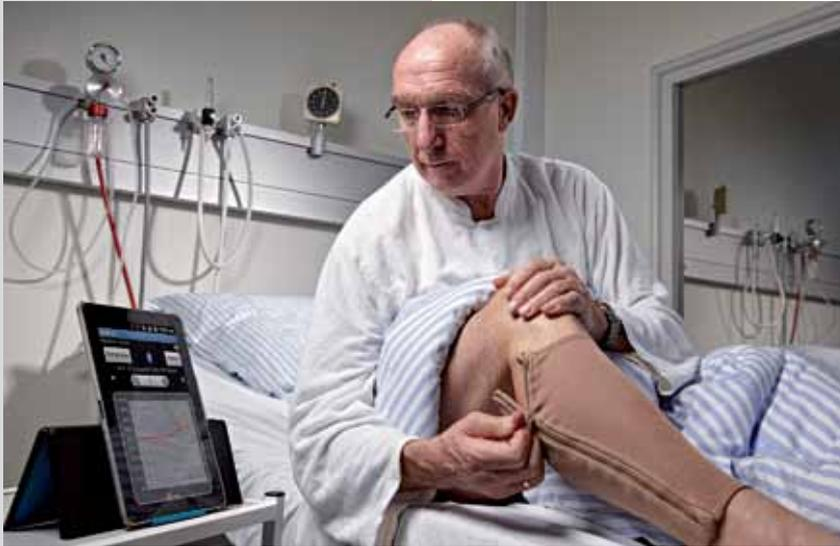
Fig. 7: Ohmatex has recently developed an Oedema sock which wirelessly measures the change in volume in the lower leg.
