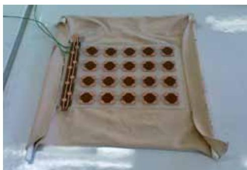
Fig. 13: RGB LED integration and OLED tile integration, both in stretch technology in combination with textile.
